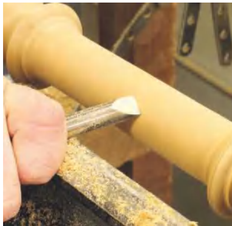
▲ Pic.23 The skew chisel is a great tool for doing planing cuts. Try and put the minimum amount of pressure down on the bevel of the tool or else you can end up with vibration marks on the stem, which you don't want
